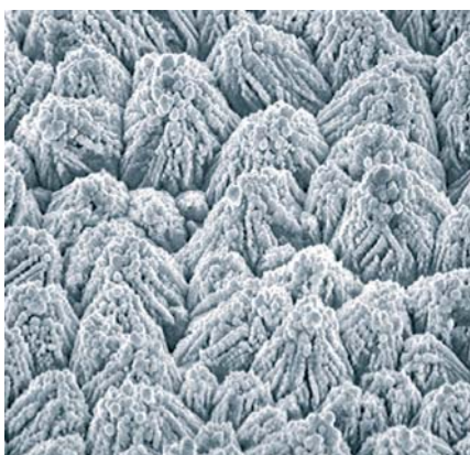
JD2HD (copper oxide treatment) and JTCHD (brass treatment, barrier layer), both 35 \mu\text{m}
